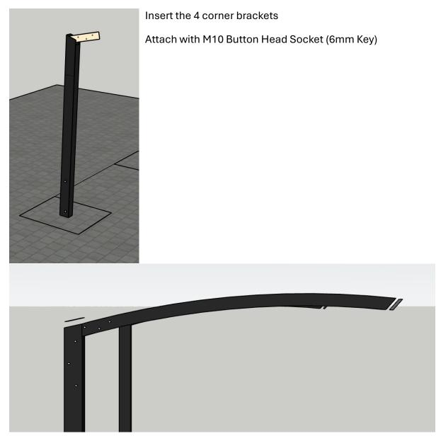
Slide rafters over corner bracket and bolt together.
